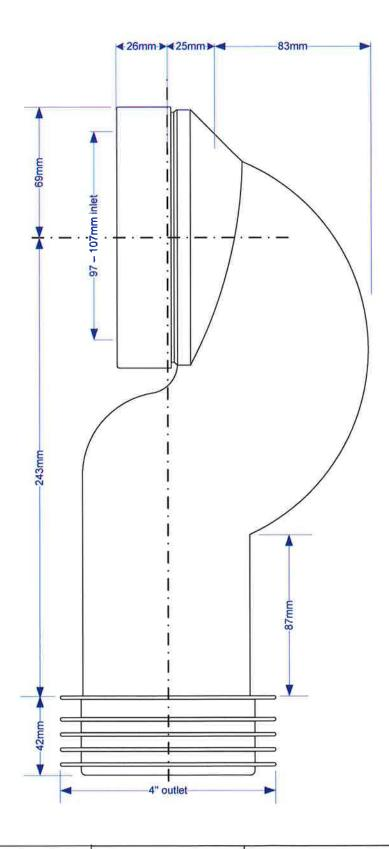
\*WC-INLET Seal has been tested to EN681
